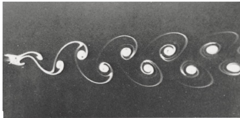
Streaklines in the unsteady flow around a cylinder. (Photograph by Sadatoshi Taneda. From Album of Fluid Motion, 1982, The Parabolic Press, Stanford, California.)
